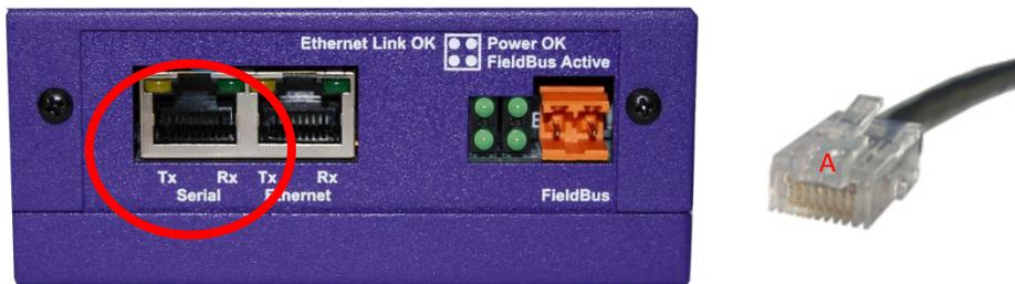
Figure 3: Serial Connection Port
