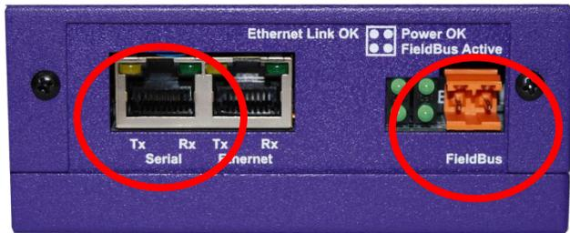
Figure 5:LonWorks Connection Ports
